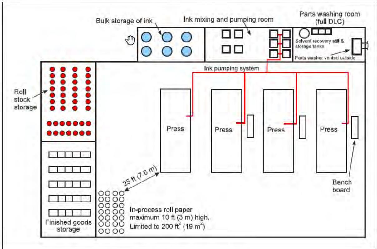
Fig. 1. Press room design and layout
