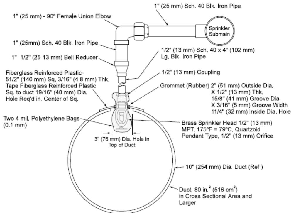
Fig. 1 - Typical sprinkler installation within a duct (Factory Mutual)
