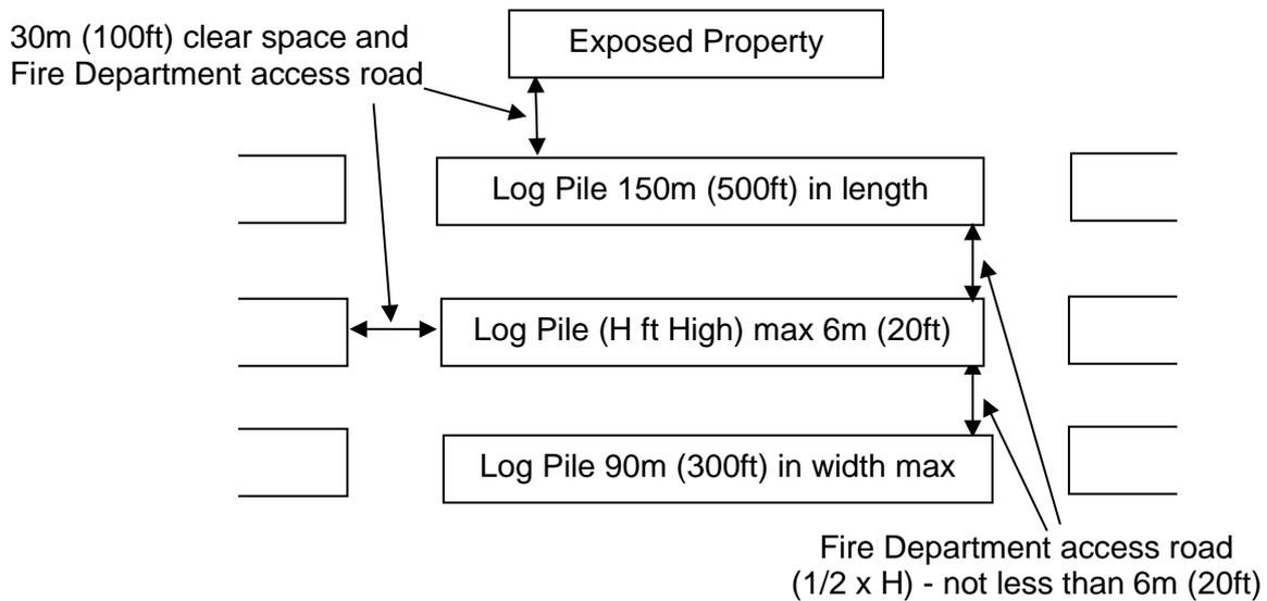
Fire lanes for access across each end, providing a clear space of at least 30m (100ft) to adjacent pile rows or other exposed property, should be provided. Where practical, greater widths are desirable to minimize the effects of radiated heat, particularly in high piled yards.
