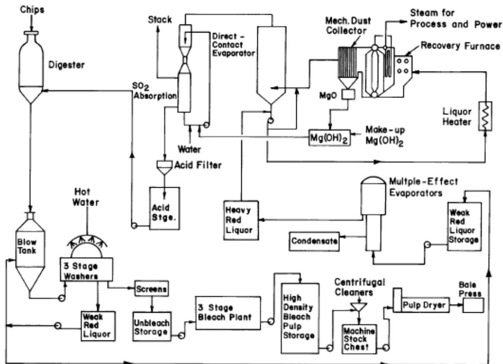
FM Global Data Sheets 7-57: Pulp and Paper Mills Fig 2 Flowchart of magnesium sulfite acid pulping and magnesium oxide recovery.
