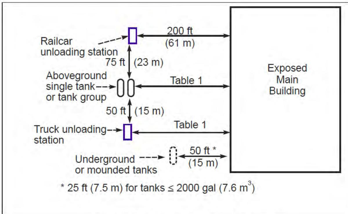
Fig. 1. Separation distances for LPG storage and unloading
