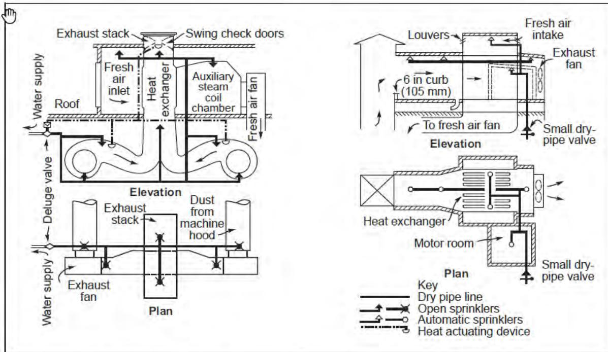
Fig. 5. Typical paper machine economizers. Suggested arrangements for automatic sprinklers.
