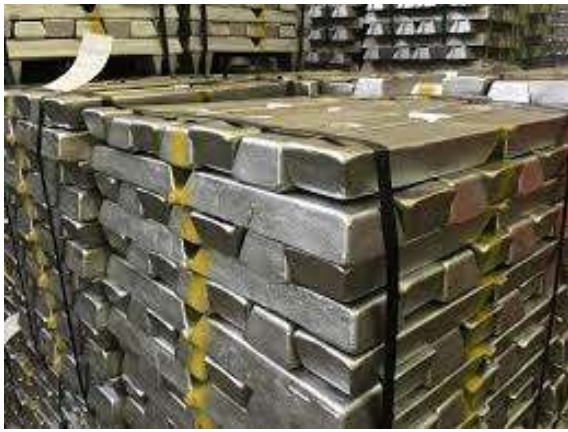
The smallest aluminum ingots, often called pigs, weigh between 6 and 24 kg
