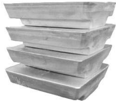
Sow ingots can weigh 700 kg and more
