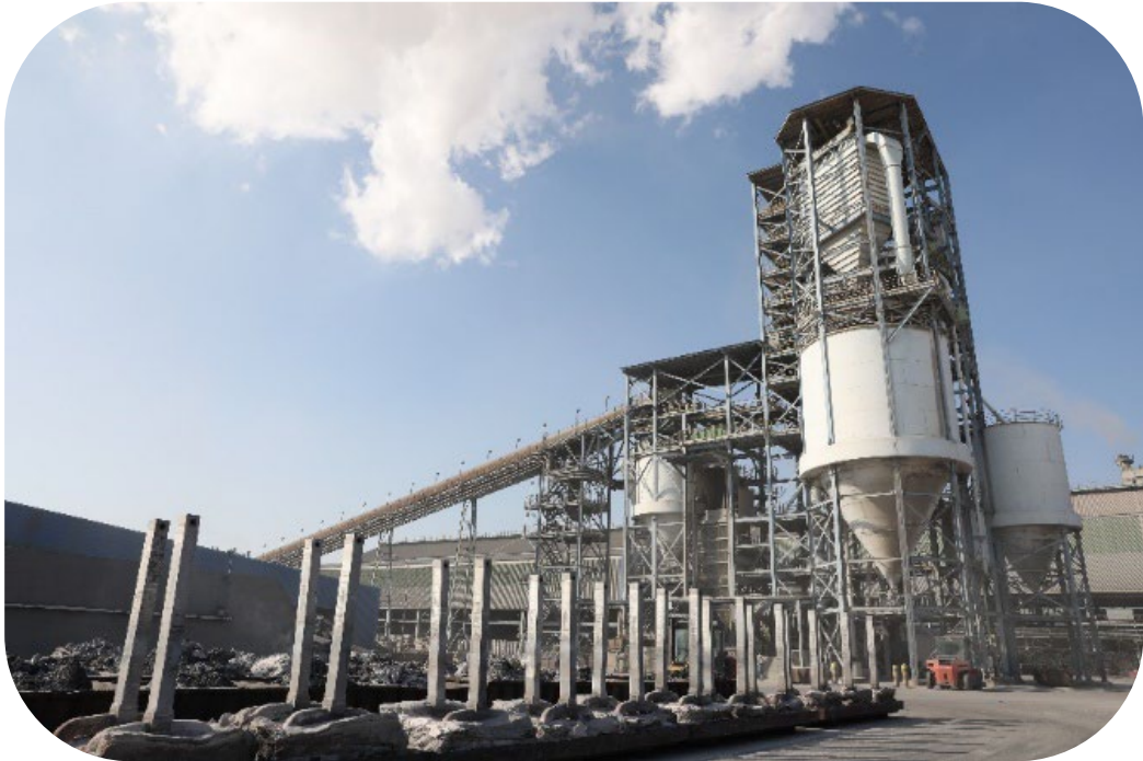
Buffer storage of rodded anodes near the cast house Courtesy of Aluminium Bahrain B.S.C. (Alba)
