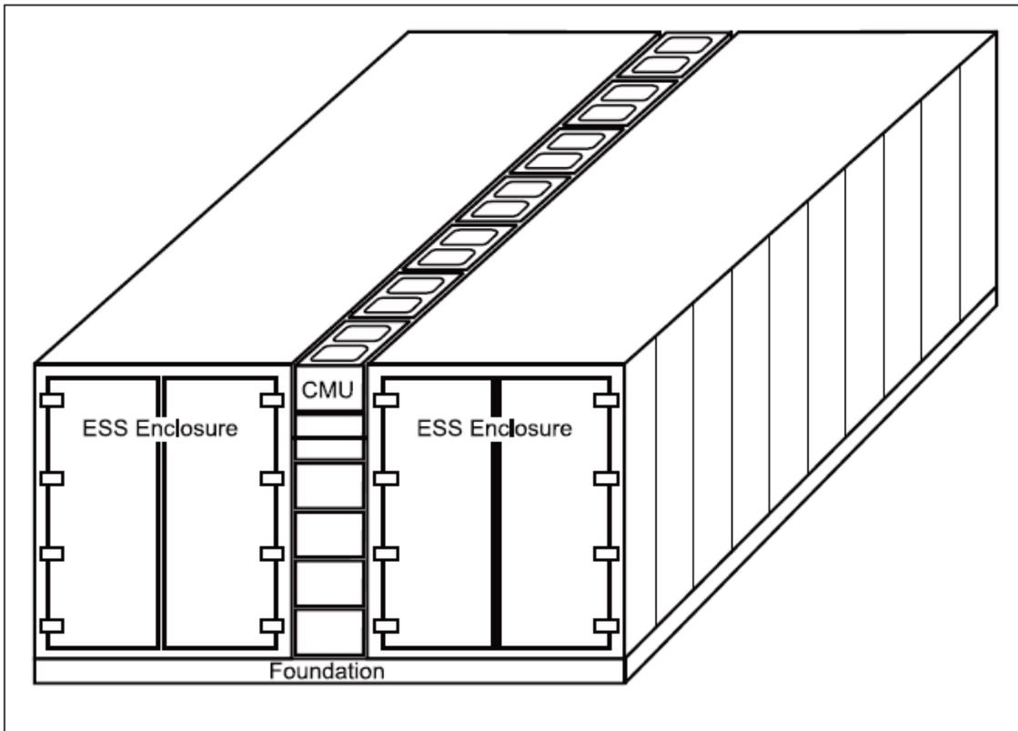
Fig. 2.3.2.2.1. Exterior ESS enclosures with fire barrier
