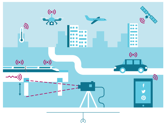
FIGURE 2: AN ILLUSTRATION OF THE RANGE OF TECHNOLOGIES WHICH CAN BE APPLIED TO MONITORING INFRASTRUCTURE, FROM SATELLITES AND DRONES TO EMBEDDED SENSING, SENSORS ON VEHICLES AND SOCIAL MEDIA DATA.
