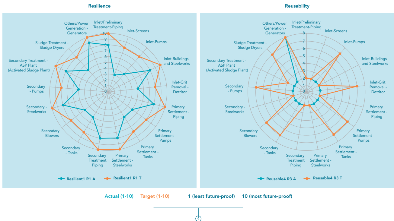
FIGURE 8: EXAMPLE RADAR PLOTS DEMONSTRATING A FUTURE-PROOFING ASSESSMENT AGAINST TWO SPECIFIC CRITERIA (AS APPLIED TO LIVERPOOL WASTE WATER TREATMENT WORKS 9 )
