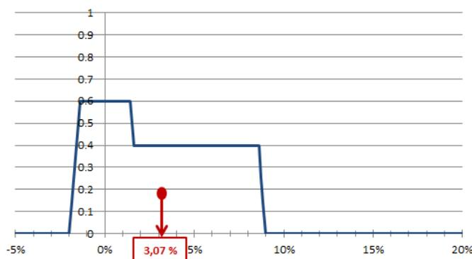
**FIGURE 17 – Defuzzification with Centre Of Gravity method**
