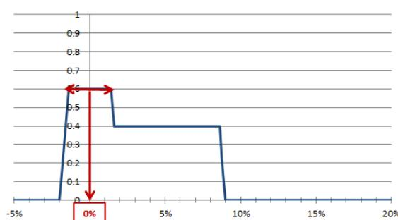
FIGURE 16 – Defuzzification with Mean of Maximum method
