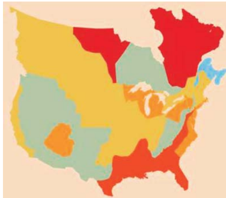
Figure 10 Relative risk from strong electric field fluctuations in the US and Canada based on ground conductivity models. Red and blue represent the highest and lowest risk regions respectively (LLoyd's & AER, 2013)
