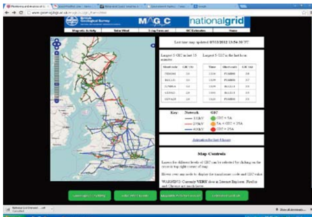
Figure 21 Real-time monitoring of GICs by National Grid (Rogers, July 2013)
