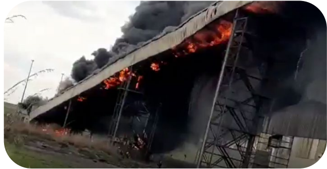
Fire on rubber belt conveyor – covered, elevated, inclined
