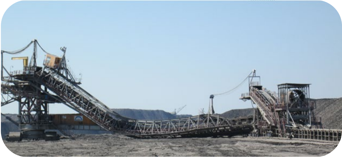
Example of conveyor collapse structures
