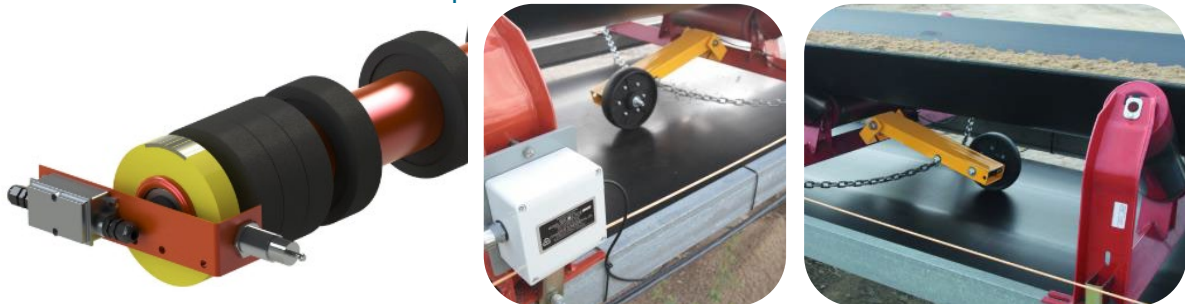
Example of belt rotation detectors
