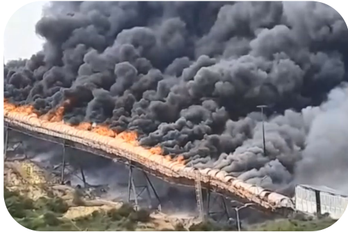
Fire on rubber belt conveyor – covered, elevated, inclined
