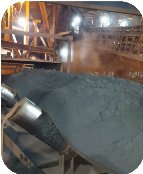
Rubber belt conveyor overload
