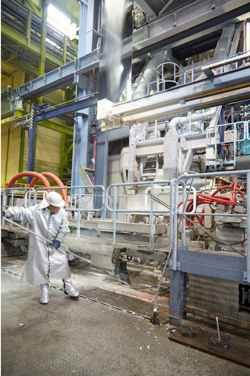
Hot Dip Galvanizing Zinc Bath - Courtesy of 'World Steel Association (worldsteel)'
