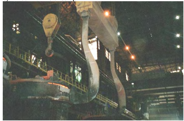
8) Pear-shaped vessel after BOF treatment ready for continuous casting
