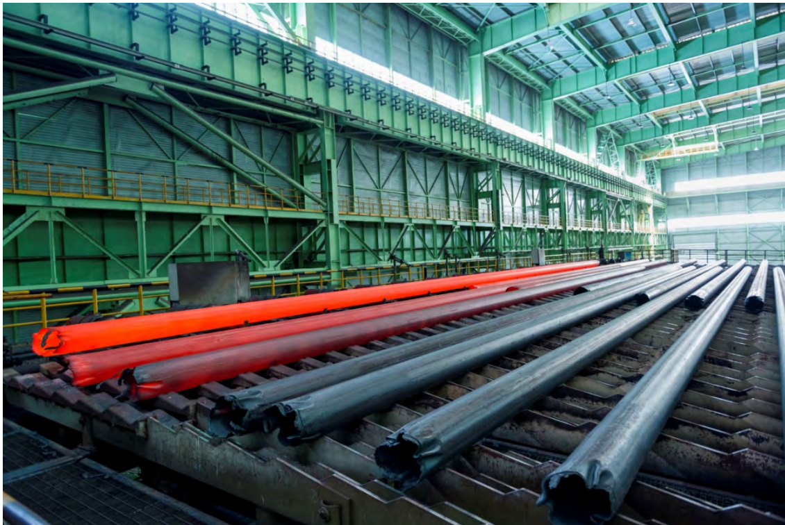
Seamless Steel Pipe on cooling bed - Courtesy of 'World Steel Association (worldsteel)'
