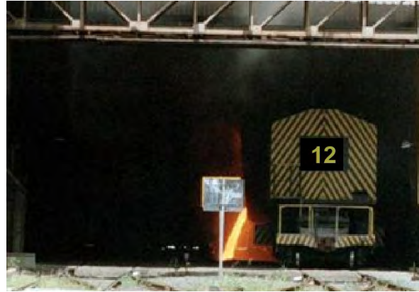
4) Pre-oxidized molten material drainage
