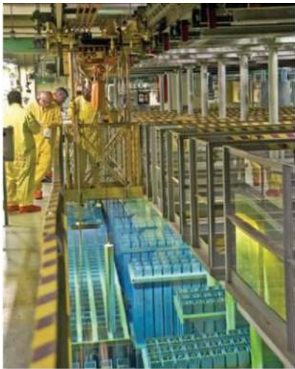
Source: DOE. Spent nuclear fuel being moved in a wet storage pool at the Savannah River Site.
